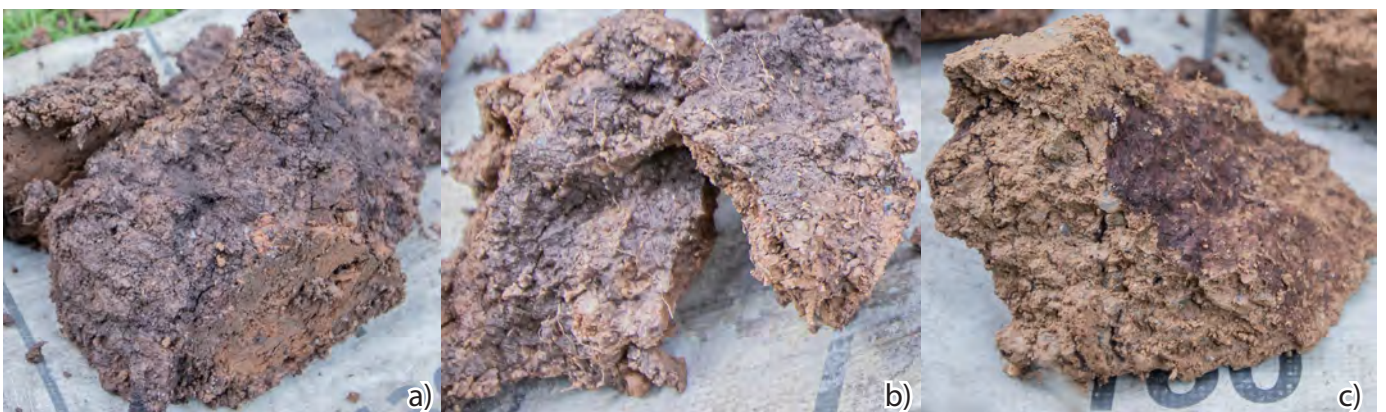
Abb. 139: Ton-Huminstoff-Cutan in RS-1 (a), in Bs-sSw (b), in sSwd (c)
